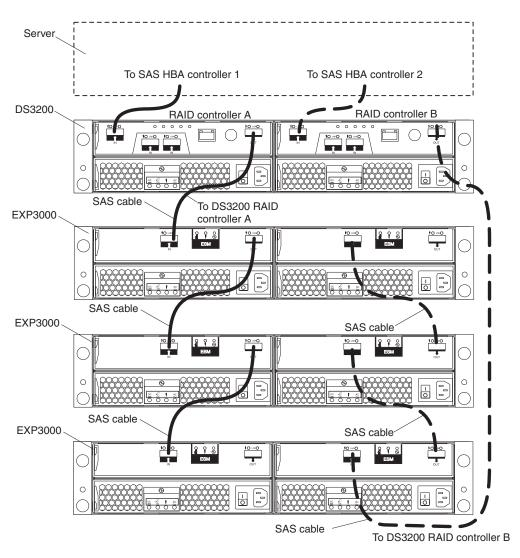
Figure 18. Example of a redundant drive path
